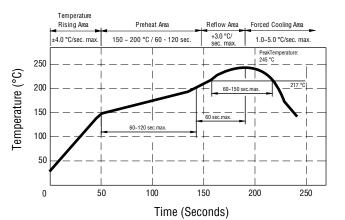
Peak Temperature: 245 ° ±5 °C max., 30 sec. max. Maximum Time Above 217 °C: 60~150 seconds
