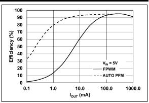
**FIGURE 2-4:** Buck1 Efficiency vs. Load Current ( $V_{OUT1} = 3.3V$ ).
