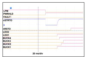
**FIGURE 2-24:** Automatic Wake-Up Pulse, Hibernate Mode.
