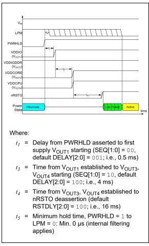
**FIGURE 4-10:** Start-Up Sequence Exiting Hibernate Mode Timing Diagram.
