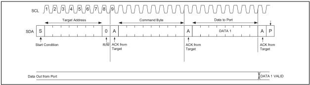
FIGURE 4-12: I<sup>2</sup>C Single Write.
