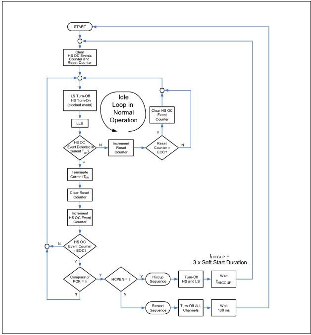
FIGURE 5-2: Hiccup Mode Protection Flowchart.
