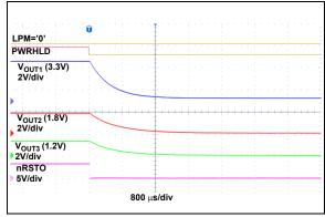
**FIGURE 2-16:** PWRHLD Shutdown Sequence.
