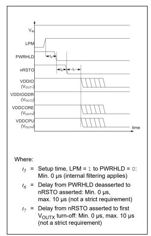
**FIGURE 4-9:** Entering Hibernate Mode Timing Diagram.
