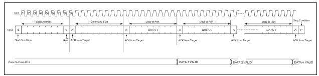
FIGURE 4-13: Block Write.
