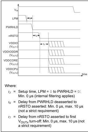
**FIGURE 4-7:** Power-Down (Shutdown) Sequence Timing Diagram.
