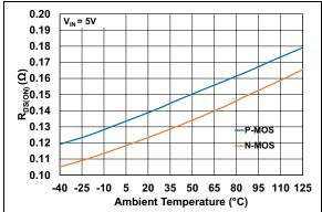
**FIGURE 2-10:** MOSFET  $R_{DS(ON)}$  vs. Temperature.
