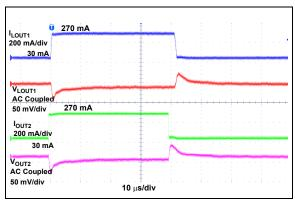
FIGURE 2-21: LDO1, LDO2 Load Transient Response.
