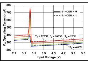
**FIGURE 2-2:**  $V_{IN}$  Quiescent Current vs. Input Voltage and Temperature – Low-Power Mode (LPM = PWRHLD = High, HPM = Low).
