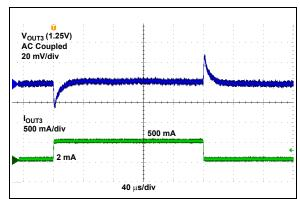
FIGURE 2-18: Buck3 Transient Response (Active Mode, V<sub>OUT3</sub> = 1.25V).
