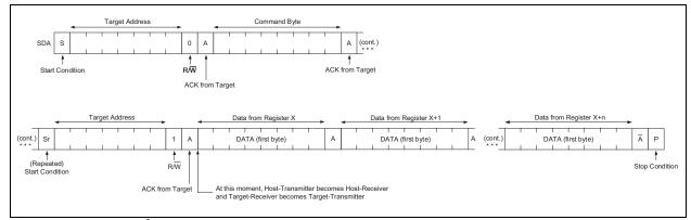
FIGURE 4-15: I<sup>2</sup>C Block Read.
