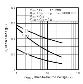
**Fig 5.** Typical Capacitance Vs. Drain-to-Source Voltage
