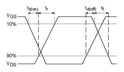
Fig 10b. Switching Time Waveforms
