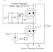
Fig 9b. Gate Charge Test Circuit
