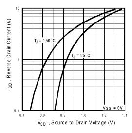
**Fig 7.** Typical Source-Drain Diode Forward Voltage
