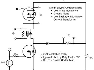
\* Reverse Polarity of D.U.T for P-Channel
