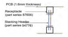
OAL = Distance between the two PCB – 7,4mm
