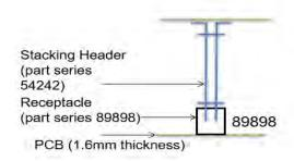
OAL = Distance between the two PCB – 2,4mm
