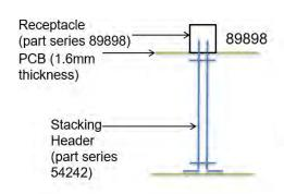
OAL = Distance between the two PCB + PCB thickness + 6,8mm
