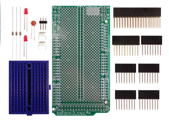
Through Hole Prototyping Shield for Arduino Mega with Components and Free Breadboard
