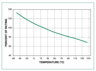
1. Re-rating depicted in this curve is in addition to the standard re-rating of 20% for continuous operation.
